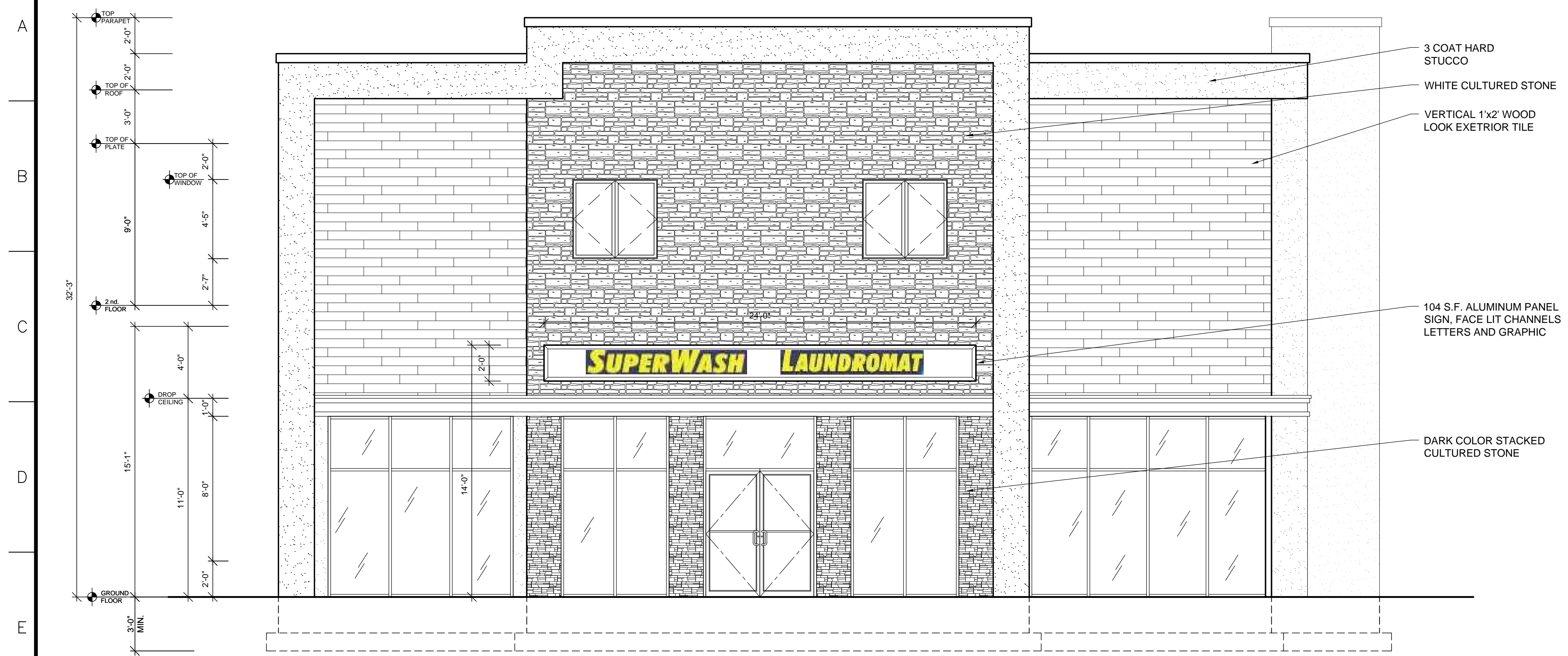
1 FRONT ELEVATION SK-4 SCALE: 1/4"=1'-0"
